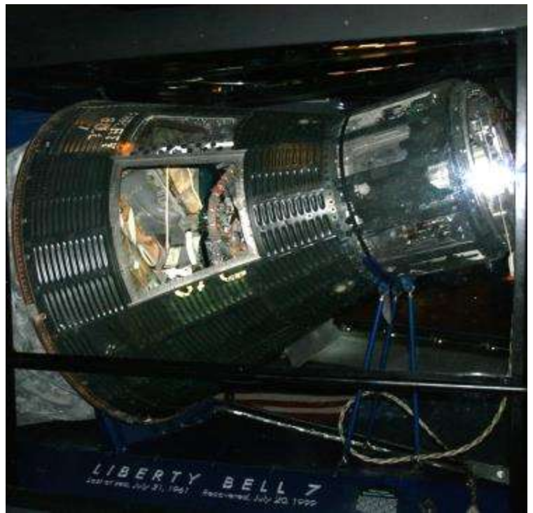
Grissom's Liberty Bell 7 now resides at the Kansas Cosmosphere in Hutchinson, KS after being retrieved from the floor of the Atlantic Ocean. You can't see it in this picture, but the hatch frame is bent. Some believe the capsule splashed down on the hatch, bending the frame and causing the hatch bolts to later fail.
