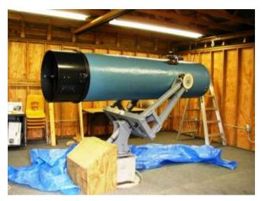
The Byers drive replaced the original drive and it makes for an interesting story. The original drive was made by Augie Wendt, an engineer at the local TV station. He used some gearing, probably from farm equipment, and wound a motor to run at the speed needed.
